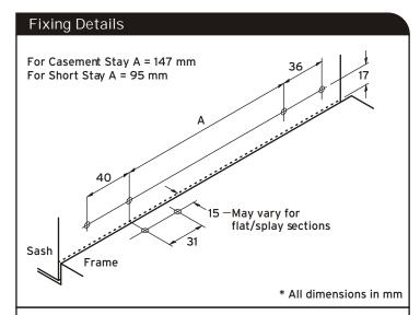
The recommended screws are No.8 Countersunk Head.
