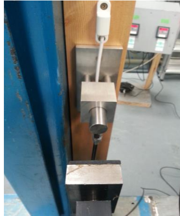
Cutting test block and restrictor mounted in test rig
