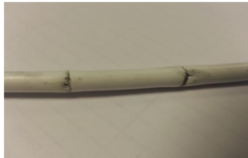
Restrictor cord after testing
