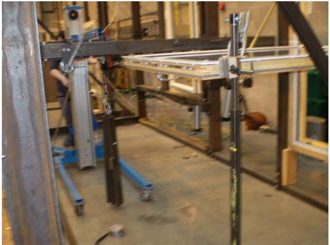
Deflection of the window during racking test
