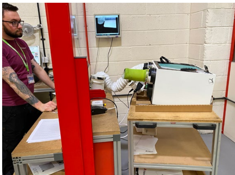
All MVHR are electronically tested
