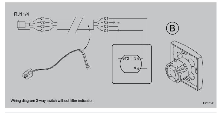
The colours of wires C1 - C6, and C1 to C4 respectively, indicated in the diagrams above may vary; that depends on the type of modular cable used.
