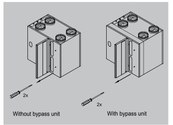
4 If the appliance is equipped with the optional bypass unit, it must now be removed.
