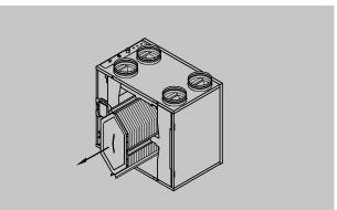
6 Clean the heat exchanger using hot water (55°C max.) and a regular detergent. Rinse the exchanger with hot water. If the appliance came ex factory with a bypass, then first remove the valve control device from the sliding grate.
