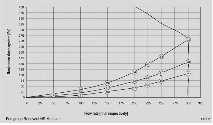
Note: The value stated in the circle is the capacity per fan (in Watt)
