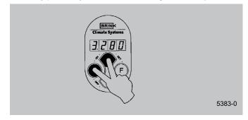
22 After cleaning the filter or a placing a new filter, the filter indication must be reset by pressing key "**OK**" during second
