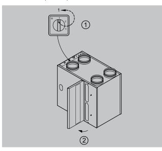
2 Remove the filters. Remember in what way the filters are taken out.
