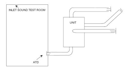
Casing breakout – the inlet and outlet ducts are connected to a separate room so the only noise measured is breakout from the casing
