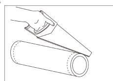
TIP: Cut each end of the tube equally to keep the external water baffle in the centre of the tube.
