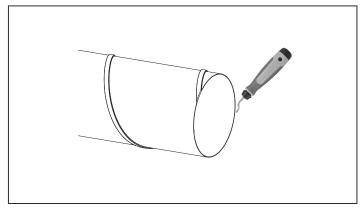
It can be cut down to suit reduced wall thicknesses and if cut to length, ensure to deburr inside edge.
