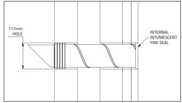
To fit the unit, push into the hole in the wall from inside the dwelling until rubber seal is in position as shown in image above. Ensure to use internal intumescent fire seal to seal between the metal ducting and internal wall.
