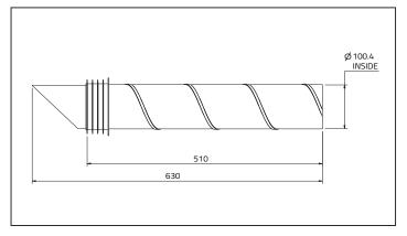
The unit is designed for a wall thickness of up to 510mm and in a 117mm hole.
